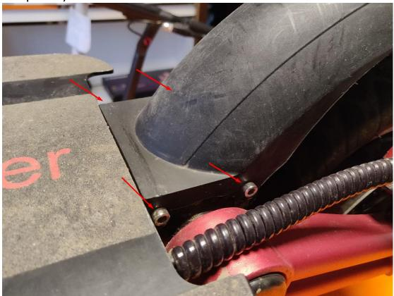
**3. a)** Tear off gently (without heating - to facilitate reassembly), sandpaper on the sides of the platform (marked in the photo), and the middle strip to the height marked with a red line (to reveal the screws).
