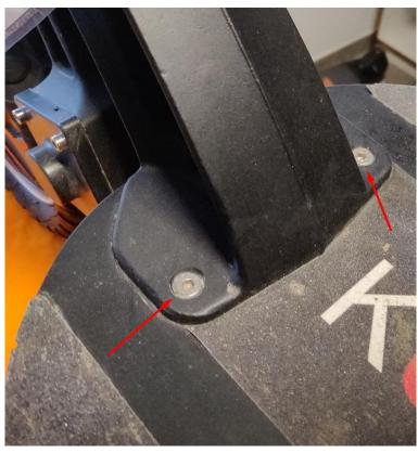
**b)** Carefully unscrew all the Allen screws under the sandpaper and those in the frame - marked in the photo.
